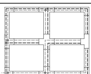
PLEASE ENSURE THAT THE DATA BUS WIRING DOES NOT CREATE A RING STRUCTURE. A FAILURE-FREE DATA BUS CANNOT BE ENSURED IF ONE IS PRESENT.
